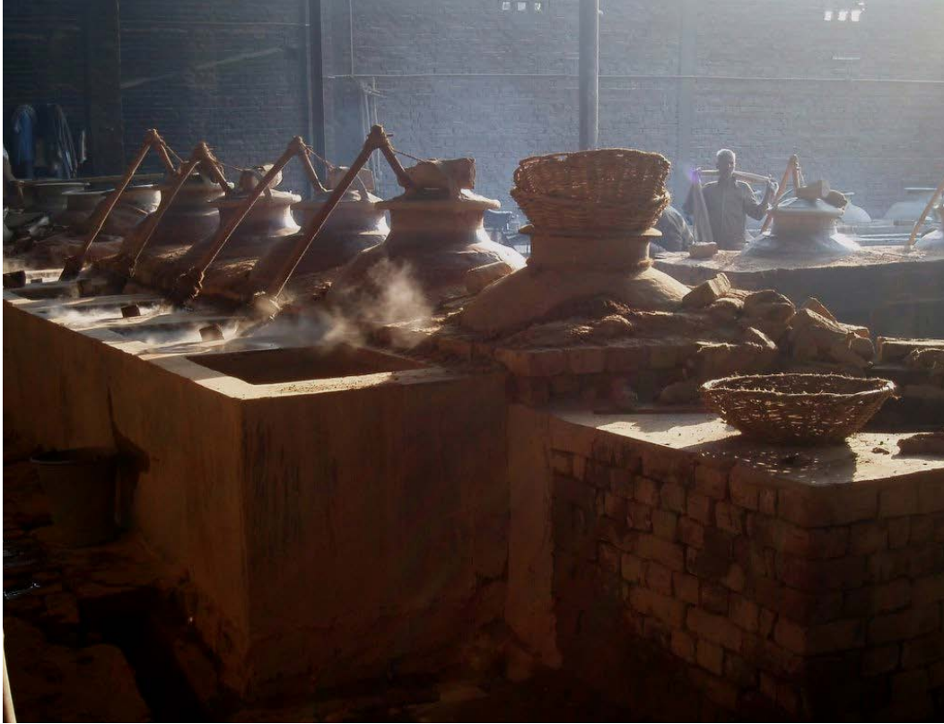
A row of Degs with bamboo pipes leading to the receiver placed in a cold-water bath at a distillery in Kannauj
