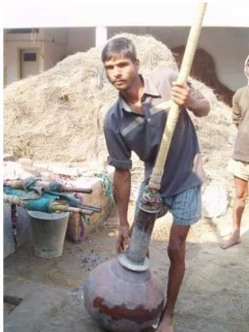
A worker prepares for the next distillation, putting the bamboo pipe in the receiver
