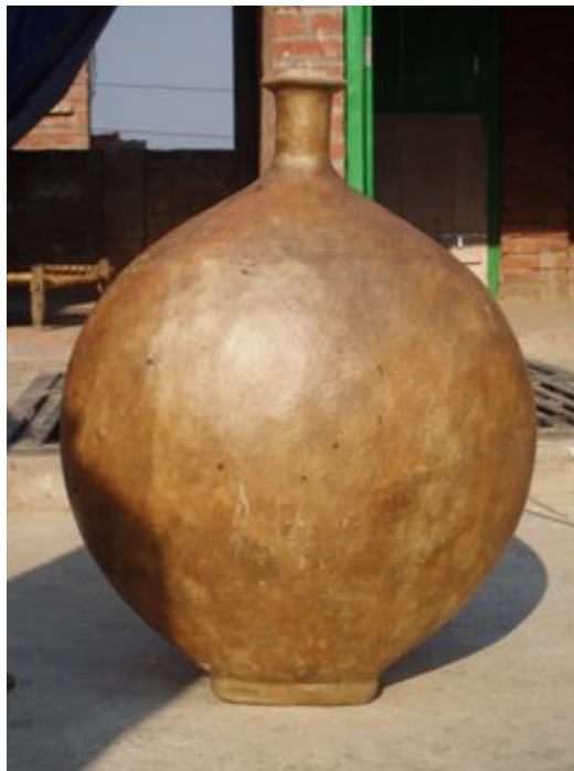
One of the leather bottles in which residual water is evaporated to form the final product
